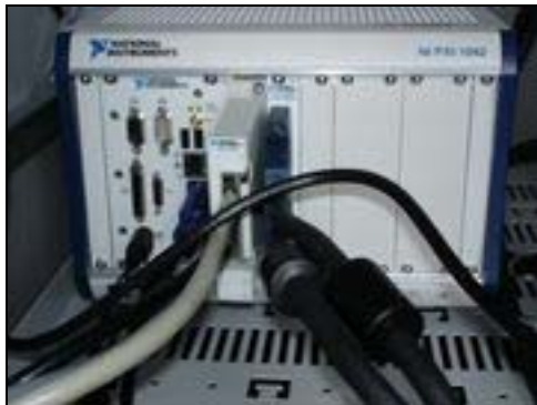
Figure 1: Controller PC: 4-channel simultaneous sampling DAQ card, 96-channel digital I/O card (National Instruments PXI-8186, PXI-6120 and PXI-6509)
